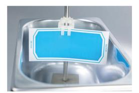
It is recommended to use these indicators at least once a day in every process used to ensure that there are no changes of the process parameters. It is also recommended to monitor each batch where loads are difficult to clean.
