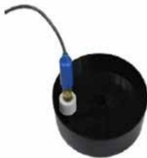
Module cable connected to 90XL display module
