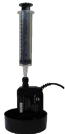
Sample tray and syringe for conductivity measurement
