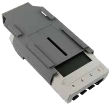
Place the Display Module in the case/holder with the screen side down as a protector
