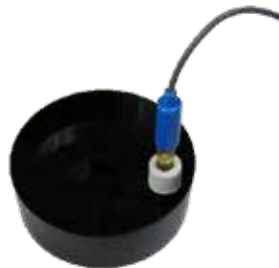
Dip sample method for pH measurement
