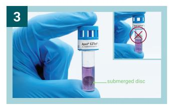
Ensure disc is completely submerged in media
