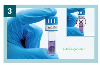
Ensure disc is completely submerged in media
