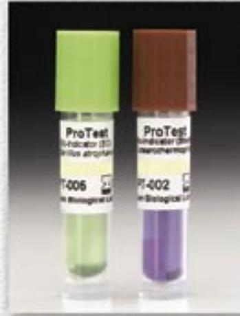
*ProTest is a self-contained Biological Indicator for use in either steam or ethylene oxide sterilization. A failed sterilization cycle is indicated by turbidity and/or a color change.*
