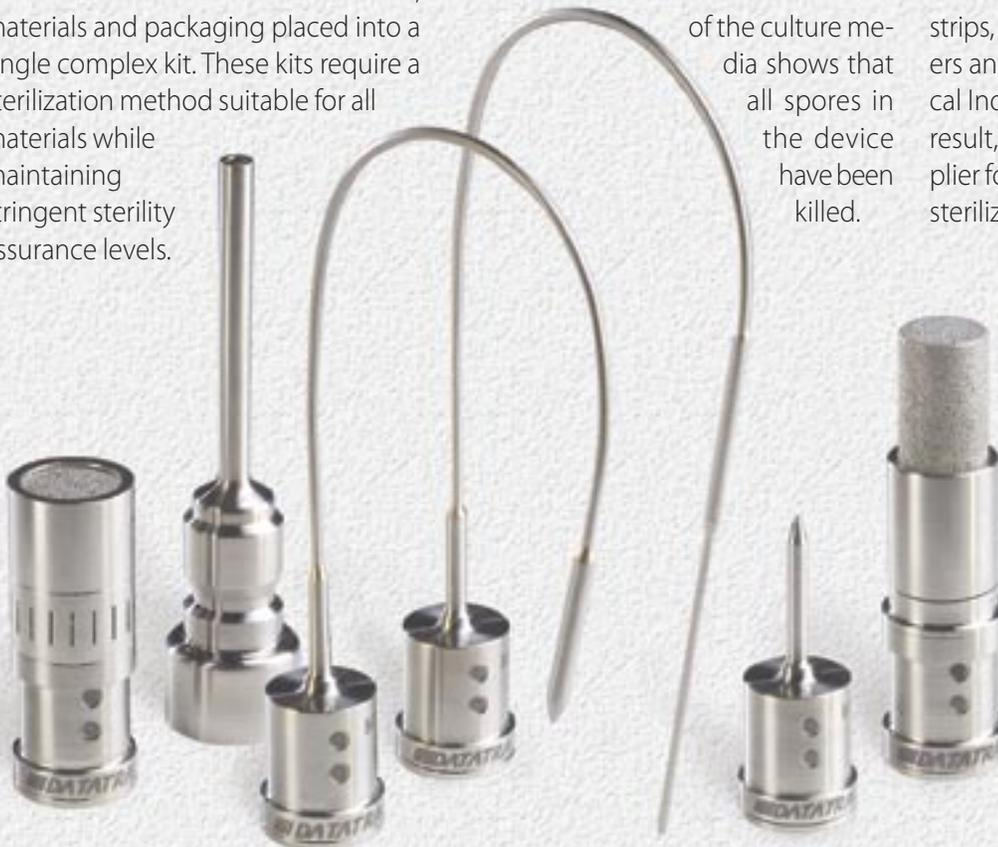
*DataTrace data loggers monitor humidity and pressure independently or in conjunction with temperature, recording as many as 16,000 individual readings before downloading.*
