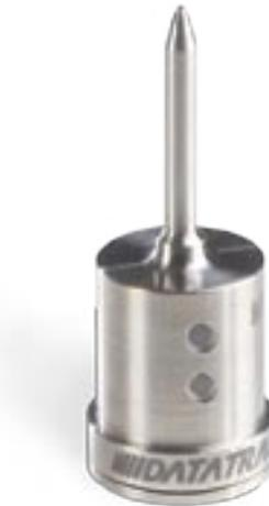
*At less than one inch in height without its probe, the Micropack III is the smallest of the DataTrace monitors with the capacity to record up to 16,000 individual readings before downloading.*
